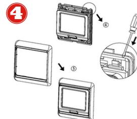
4 Install the housing cover and lock the external frame
