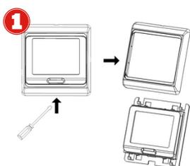
1 Release the front cover by inserting a screwdriver into bottom crack
