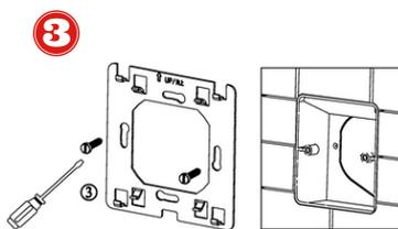
3 Install the thermostat into the electrical connection box with screws
